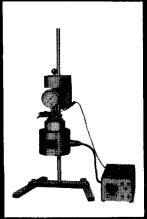
Provide all of the facilities needed for applying heat, pressure and agitation to a wide variety of chemical operations at pressures to 2000 psig and temperatures to 350° C.
